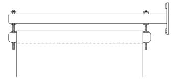
To change banners the locknuts and nuts are loosened off to remove tension from banners so that the tension arms can be slid out, the new banner is then attached and can be tensioned up with same procedure in reverse.
